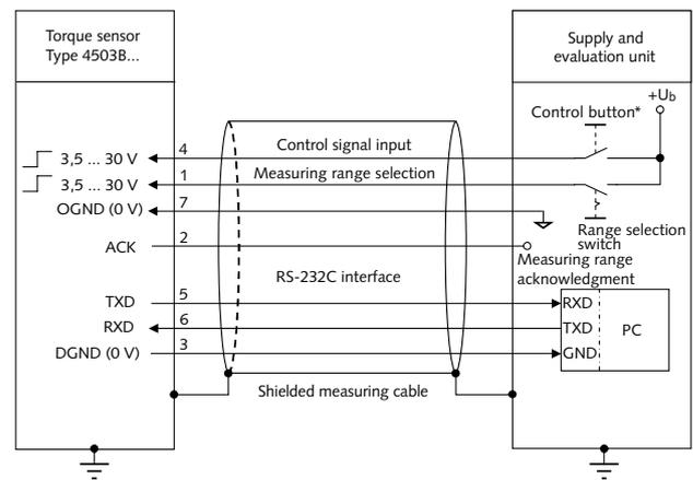
Fig. 6: Connection diagram of 7 pin built-in connector
