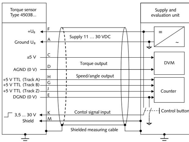
Fig. 5: Connection diagram of 12 pin built-in connector (standard)
