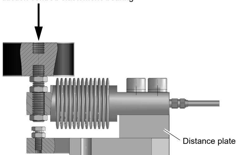
The illustration below schematically represents the correct central load introduction. Below it, examples of incorrect loading conditions are shown, which must be strictly avoided. The following points must be observed during
