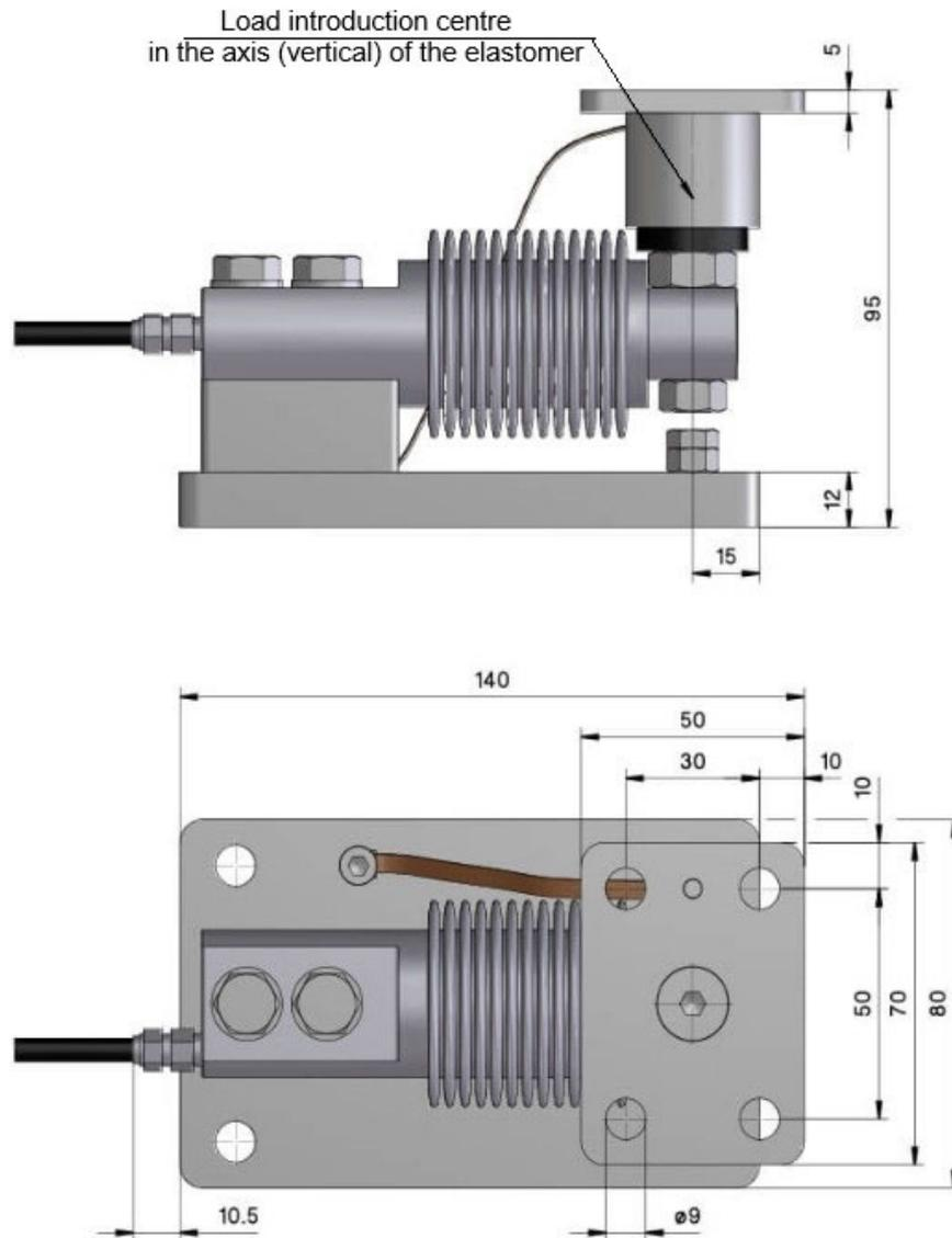
Abmessungen in mm
