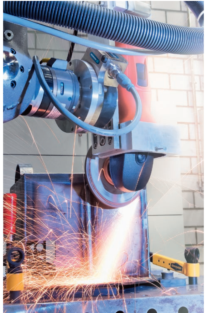
The force/torque feedback between the robot and SCHUNK FT sensor allows a significantly increase in quality of the automated grinding of supply air chambers for fireplaces.
